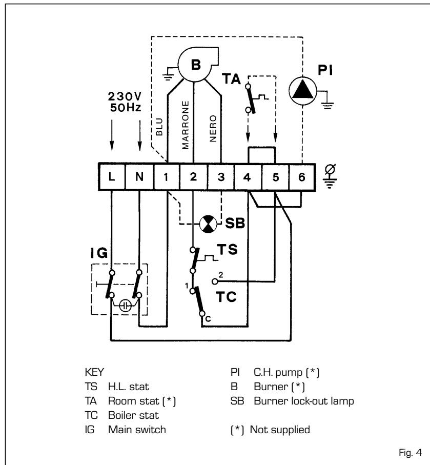
the main switch protected by fuses. The room thermostat (required for enhanced room temperature control) should be installed as shown in fig. 4. Connect the burner power cables
